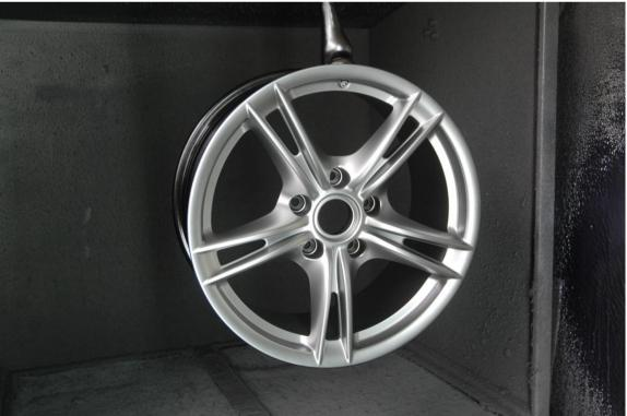
Back in the oven, which is raised from the 50 degree wet colour application to 200 degrees, once this has been reached all 4 wheels are lacquered with a Dry Powder clear gloss coat and a Final bake
