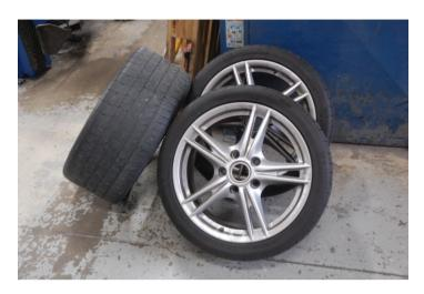
This set had succumbed to the water that sits in the valve hole and eats away the thin layers of OE paint, which up to 150 microns is the aim for OE done by Robots, TWR's finished paint thickness has been measured at 2.5 - 3 times thicker than this.
