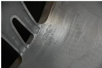
With the 3 Coat system the 1<sup>st</sup> coat (A thick dry Powder Primer) can be used to flat Down by hand these surfaces to eradicate the pitting marks, time consuming but the final results are always well worth doing this.
