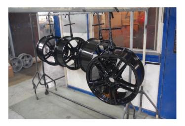
The Black colour hides any irregularities to the surface until the surfaces are Sanded by hand (Paper) to show up what needs attention (Pitting & an Orange peel finish)
